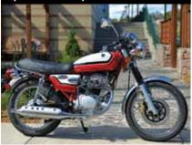
The air-cooled, 150cc, four-stroke single is a modern interpretation of Honda's stonesimple CB125. It produces almost 15 horsepower, enough for a 65 mph top speed.
